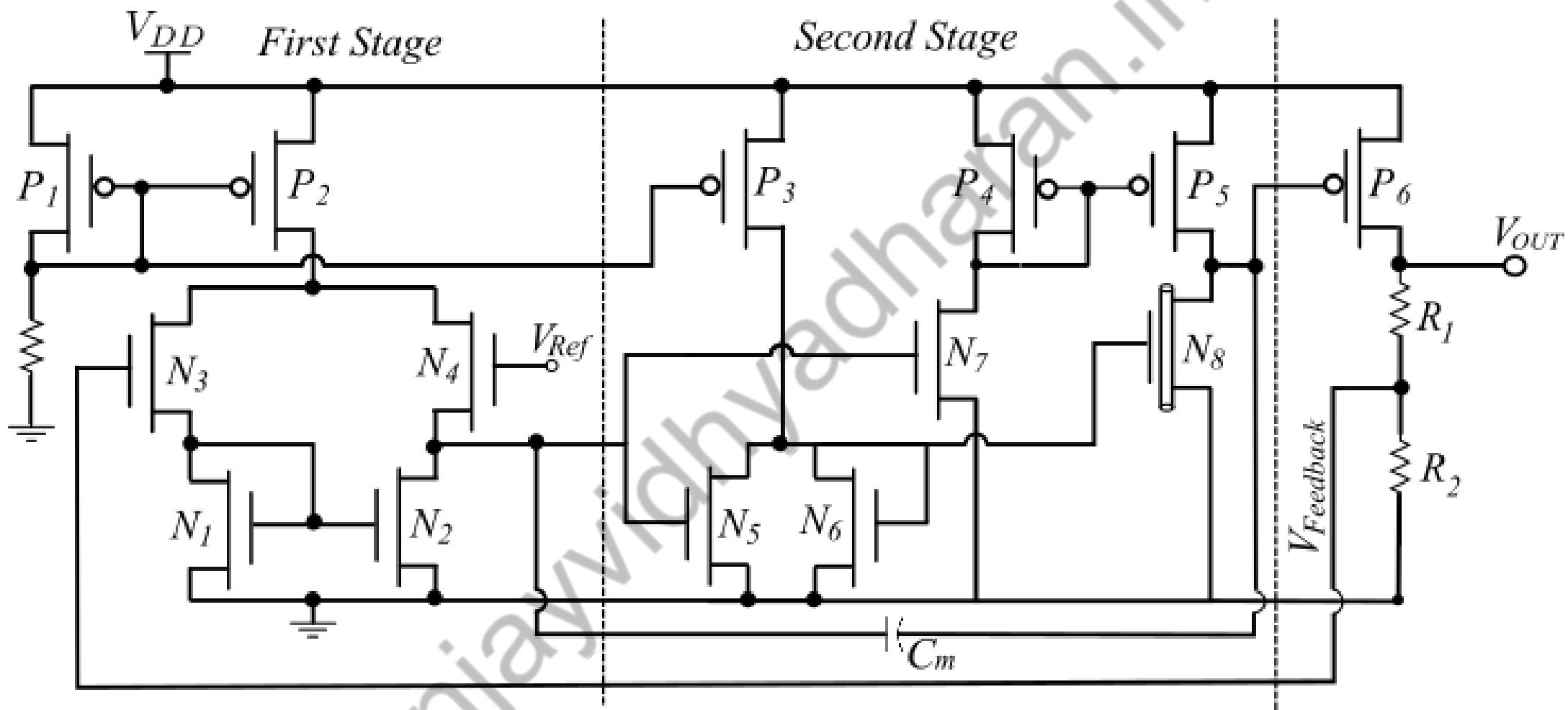
$$\frac{V_{out} * R_2}{R_1 + R_2} = V_{Ref}$$
