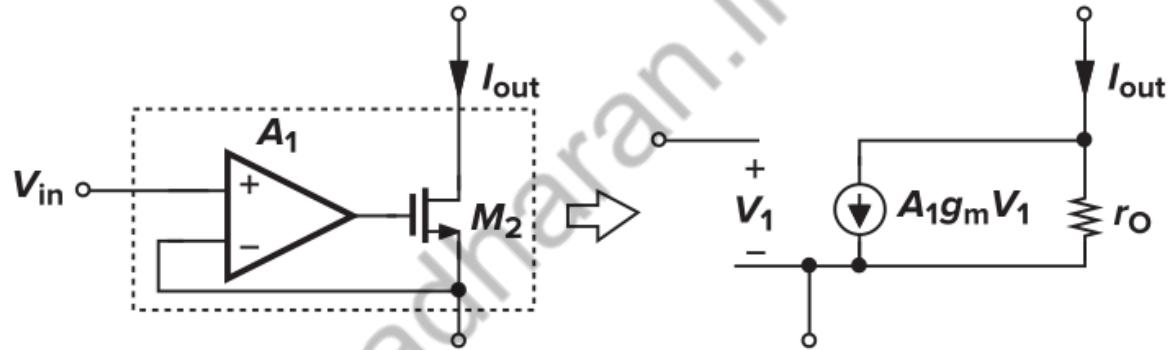
The idea behind gain boosting is to further increase the output impedance without adding more cascode devices.
