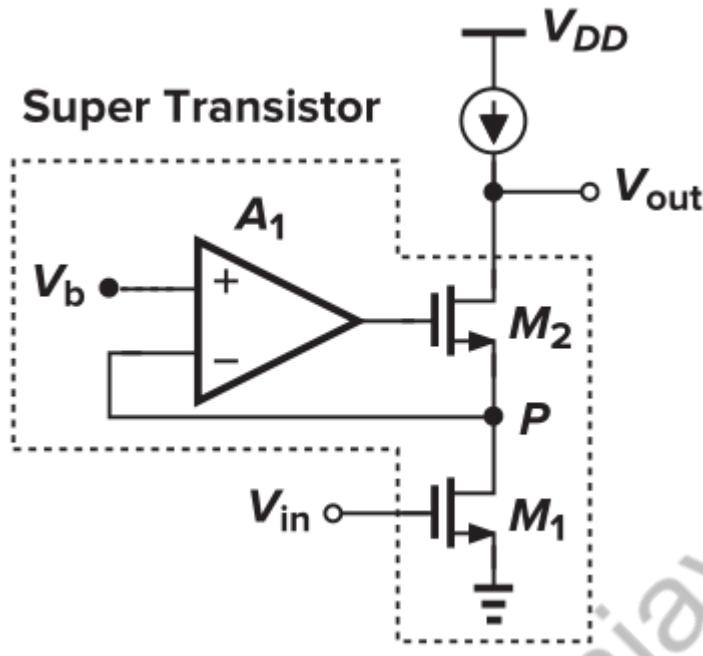
$$V_p \approx V_{in} \quad (g_{m1} \approx g_{m2})$$
