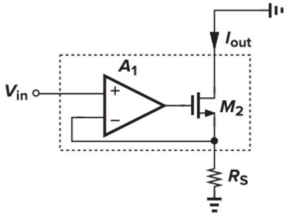
$$V_d = V_{in} - I_{out}R_s$$
