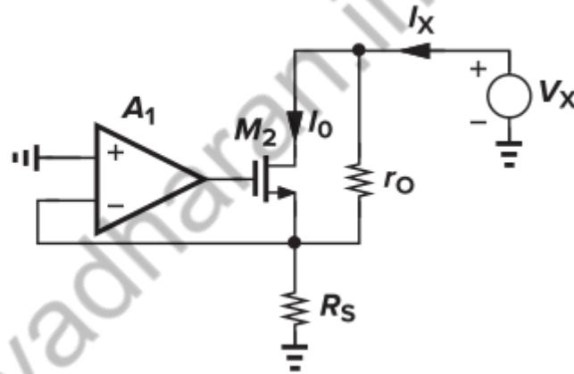
$$I_X = (-A_1 R_s - R_s)g_m I_X + \frac{V_x - R_s I_X}{r_o}$$
