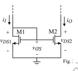
Assume that  $v_{DS2} > v_{GS} - V_{T2}$ , then
