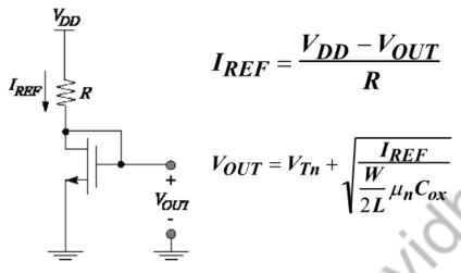
For large W/L:  $I_{REF} pprox rac{V_{DD} - V_{Tn}}{R}$
