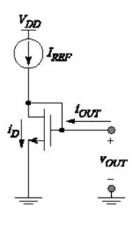
$V_{GS} = V_{DS}$  takes a value needed to sink current
