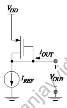
Same operation and characteristics as NMOS voltage source. PMOS needs to be larger to attain the same Rout .
