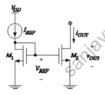
$$I_{OUT} \approx \frac{1}{2} \left(\frac{W}{L}\right)_{2} \mu_{n} C_{ox} (V_{REF} - V_{Tn})^{2}$$
