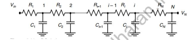
$$\tau_{Di} = C_1 R_1 + C_2 (R_1 + R_2) + \dots + C_i (R_1 + R_2 + \dots + R_i)$$
