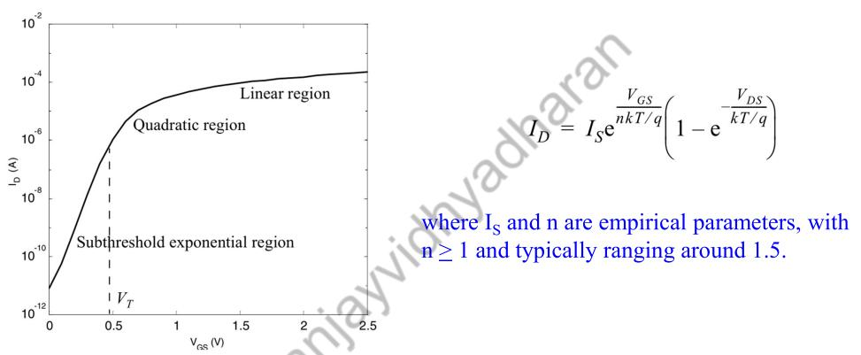
Subthreshold current has some important repercussions. In general, we want the current through the transistor to be as close as possible to zero at  $V_{GS} = 0$ . This is especially important in the so-called dynamic circuits, which rely on the storage of charge on a capacitor and whose operation can be severely degraded by subthreshold leakage.
