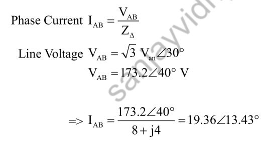
A balanced positive sequence Y-connected source with  $V_{an} = 100 \angle 10^{\circ}$  V is connected to a  $\Delta$ -connected balanced load with impedance  $(8 + j4) \Omega$  per phase.
