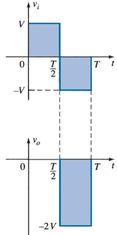
Input and Output voltage waveform
