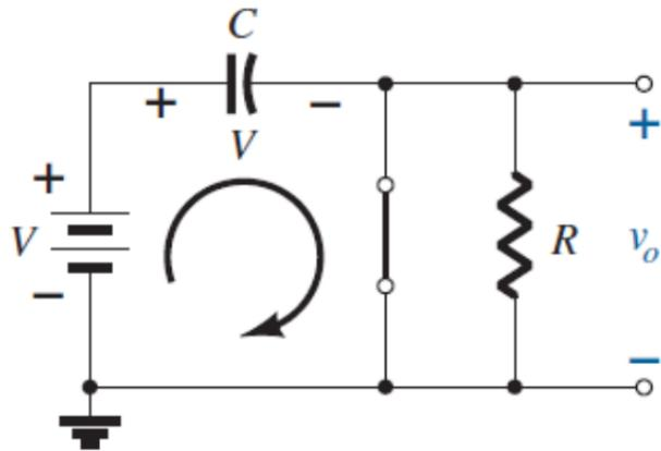
Circuit during Diode ON
