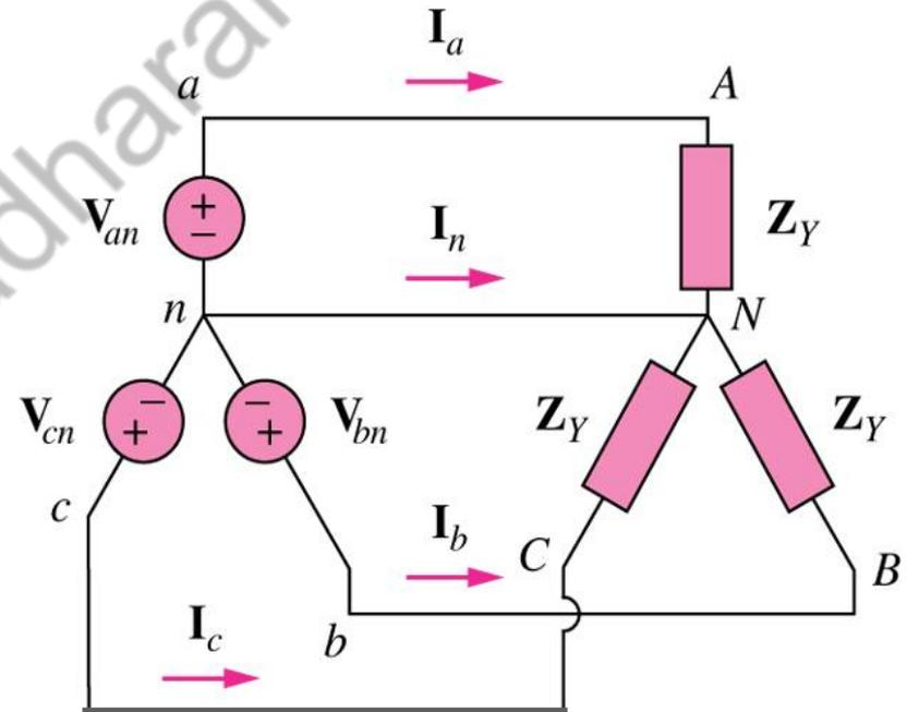
The line current is the current in each line, the phase current is the current in each phase of the source or load.
