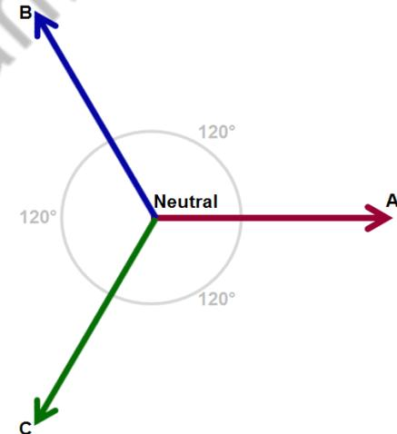
Phase voltages: voltages between lines a, b, and c and the neutral line n ( $V_{an}$ ,  $V_{bn}$ , and  $V_{cn}$ ).
