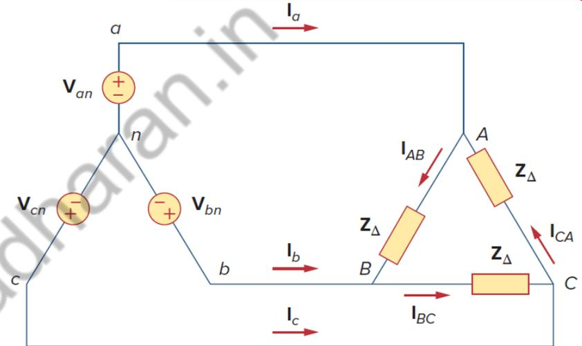
$$I_a = I_{AB} - I_{CA}, I_b = I_{BC} - I_{AB}, I_c = I_{CA} - I_{BC}$$
