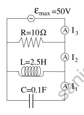
$$X_R \doteq R = 10\Omega, \quad X_L \doteq \omega L = 10\Omega, \quad X_C \doteq \frac{1}{\omega C} = 2.5\Omega.$$
