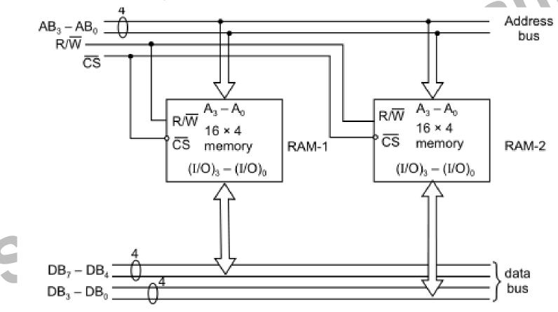
Develop a  $32 \times 4$  memory module by combining two  $16 \times 4$ memory chips. Draw the Schematic showing the Address nd ection to satisfications satisfications satisfications Bus, Data Bus and Chip Select Lines Connection to the
