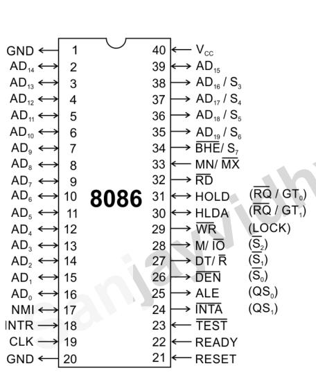
The 8086 microprocessor can work in two modes of operations: Minimum mode and Maximum mode.
