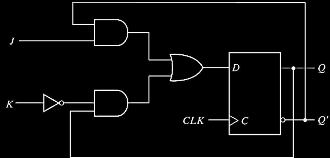
Design J-K Flip-flop using D flip-flop
