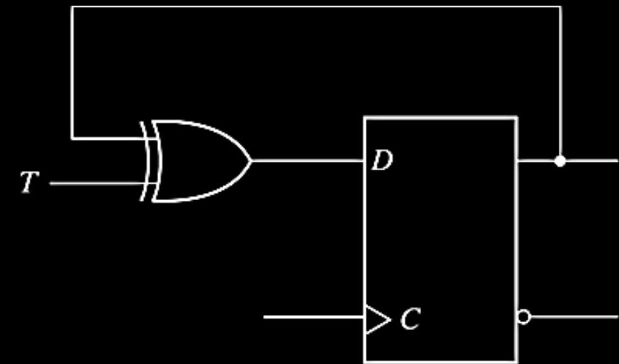
Design T Flip-flop using D flip-flop
