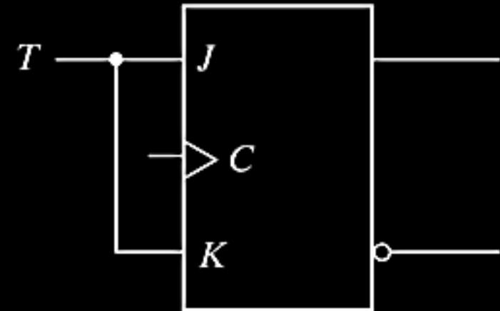
Design T Flip-flop using JK flip-flop
