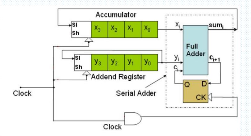
Block Diagram of a 4-bit Serial Adder with Accumulator
