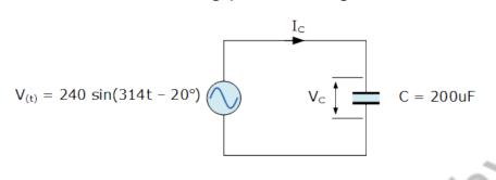
$$X_{C} = \frac{1}{j\omega C} = \frac{1}{314 \times 200 \mu F} = 16 \angle -90^{\circ}$$
