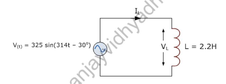
The rms voltage across the coil will be the same as from the supply voltage. If the power supplies peak voltage is 325V, then the equivalent rms value will be 230V. Converting this time domain value into its polar form gives us:  $V_L = 230 \angle -30^\circ$  (volts). The inductive reactance of the coil is:  $X_L = \omega L = 314 \times 2.2 = 690\Omega$ . Then the RMS current flowing through the coil can be found using Ohms law as:
