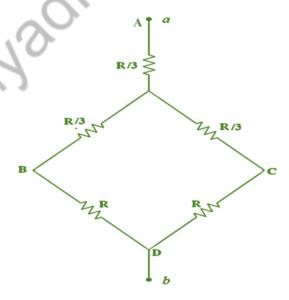
Obtain the equivalent resistance  $R_{ab}$  for the circuit and use it to find current i.
