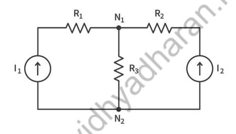
$R_1 = 10 \quad \ R_2 = 20 \quad \ R_3 = 30 \quad \ I_1 = 1A \quad \ I_2 = 2A$
