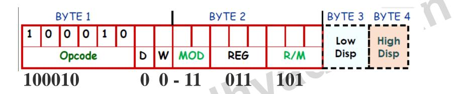
MOV = Move Register/Memory to/from Register Immediate to Register/Memory 76543210 100010 dw 1100011 w
