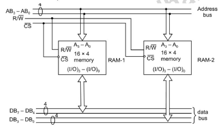
Develop a 32 × 4 memory module by combining two 16 × 4 memory chips. Draw the Schematic showing the Address Bus , Data Bus and Chip Select Lines Connection to the Chip.
